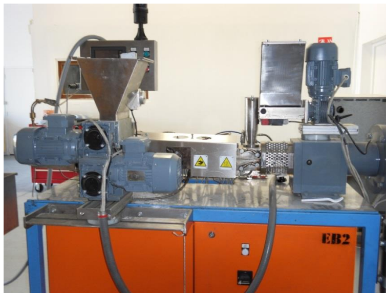
Figure 71: Extrudeuse bi-vis co-rotative TSA FSCM 21-50 (Source : Natureplast)
